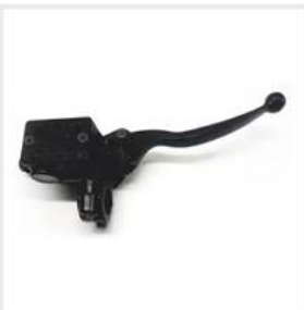
BOMBA5** BOMBA FRENO C/ MANIJA YAMAHA CRYPTON
